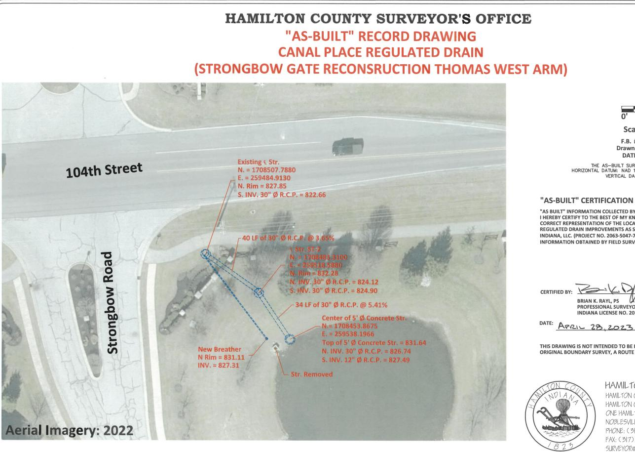
S:\E-SURV\PROJECTS\SUBDIVISIONS\CANAL PLACE DRAIN\DWG\As\_Built\_Canal Place Drain.dwg
